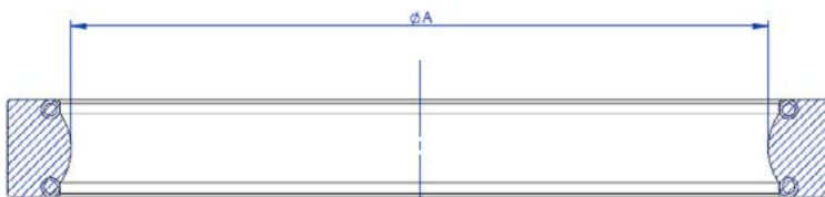
Internal Diameter (A) of Rod Type Spring Seal
